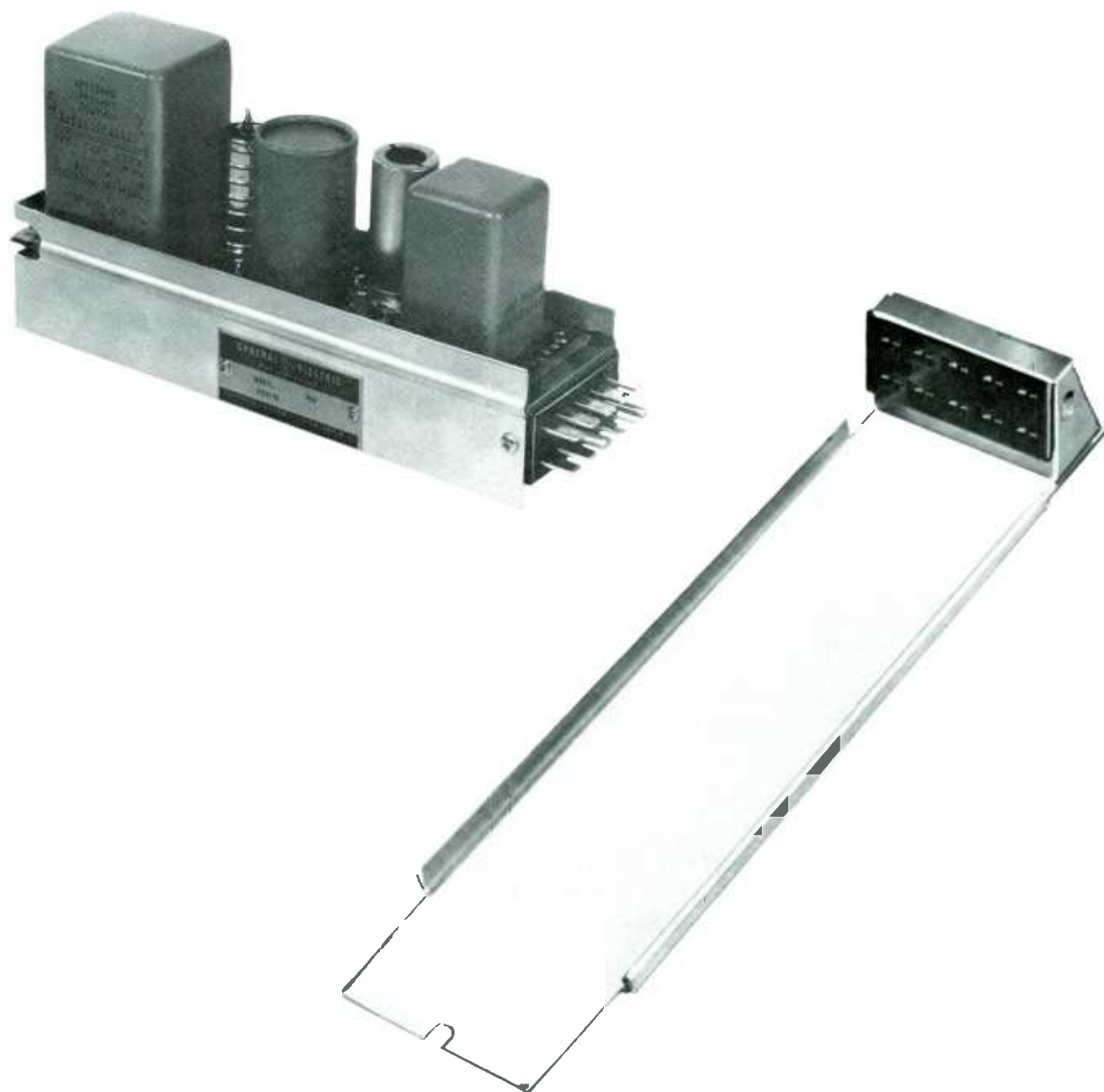
Type BA-1-H Plug-In Pre-Amplifier, Type FA-22-D Tray
