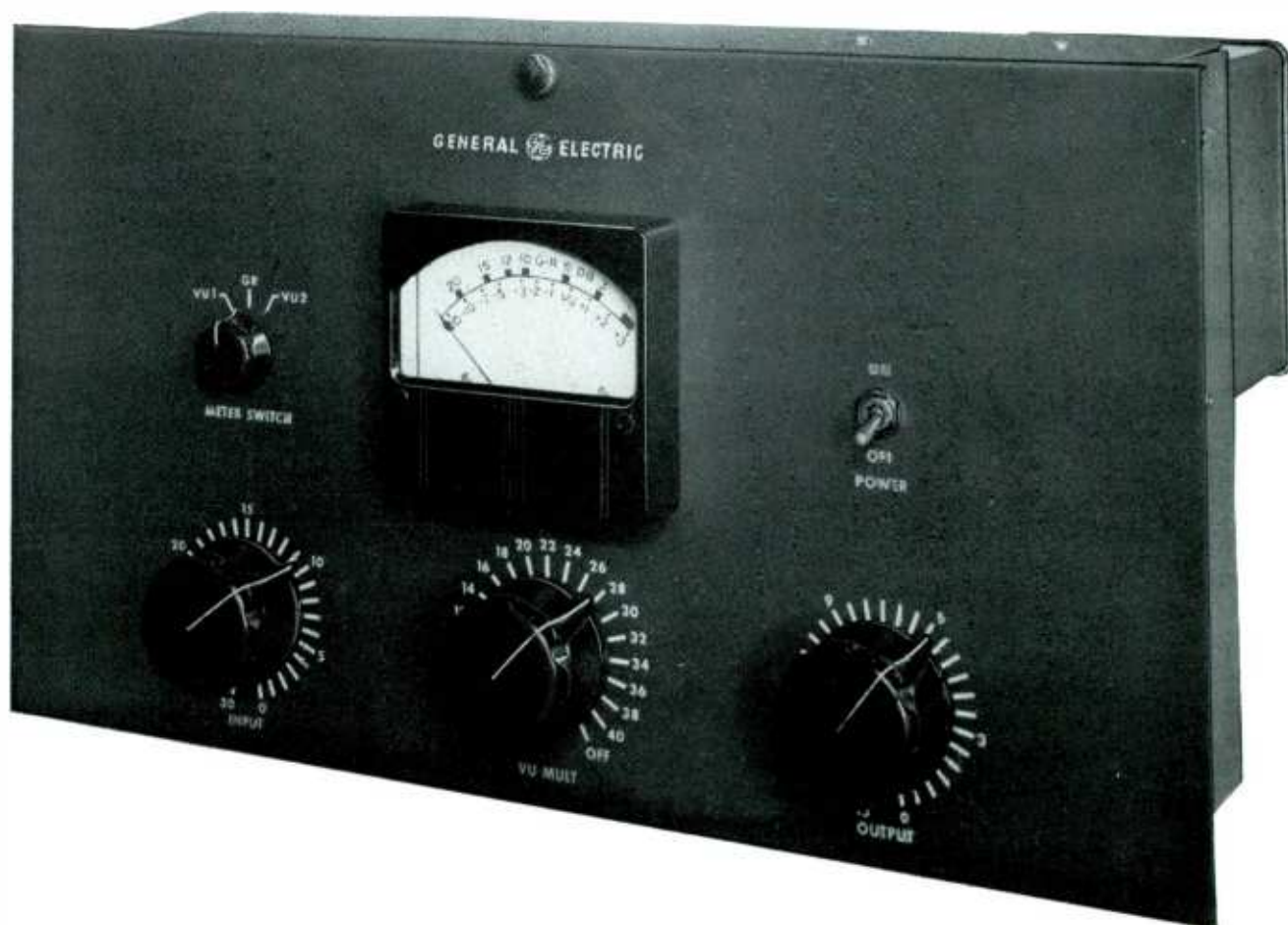
Type BA-7-A Audiomatic Limiting Amplifier
